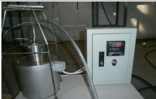
Lab-scale pyrolysis at the Faculty of Engineering
